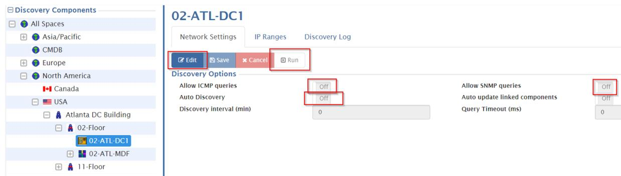
3. Switch both **Allow ICMP queries** and **Allow SNMP queries** to **On**
